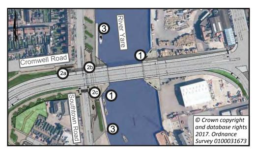
The new bridge needs to open to allow the passage of boats and large vessels along the river. The Stage 2 Consultations in Summer 2017 helped confirm our view that the best solution for an opening bridge is to provide a bascule bridge with two sections or 'leaves' that lift. The bridge would have a clearance of 4.5m over the water at high tide when in the lowered position.
