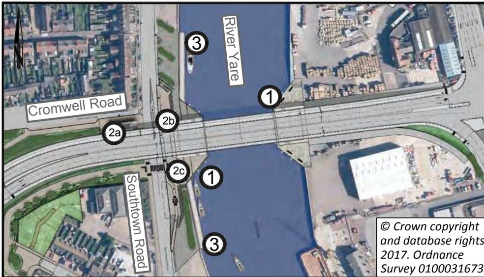
The new bridge needs to open to allow the passage of boats and large vessels along the river. The Stage 2 Consultations in Summer 2017 helped confirm our view that the best solution for an opening bridge is to provide a bascule bridge with two sections or 'leaves' that lift. The bridge would have a clearance of 4.5m over the water at high tide when in the lowered position.
