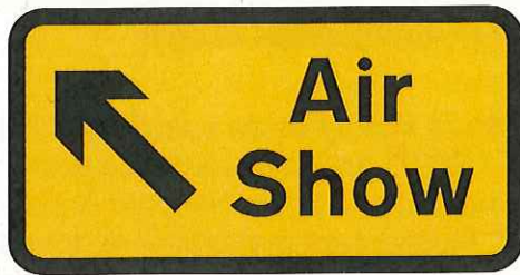
Example of an advance direction sign (ADS).
