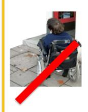
Paths should be as level as possible, with drainage. They should be at least 1.5 metres wide and even and slip resistant. Drops should be avoided or have a guard.
