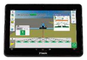
106647 Precision Input Management, based in Suffield, was contracted in January 2018. The Wensum & Coast LAG is supporting the purchase of a Trimble TMX system, a satellite receiving system allowing precision application of seed fertiliser and spray, to fit onto existing farm machinery.
